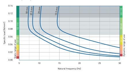
Natural frequency of a single-degree-offreedom system consisting of a fixed mass and an elastic bearing consisting of PURASYS vibrafoam SD 65 on a stiff subgrade.
