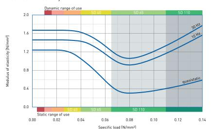
Dynamic test: sinusoidal excitation with an oscillating range of ± 0.22 mm at 10 Hz and  $\pm$  0.08 mm at 30 Hz
