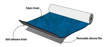
FONOSTOPTIle Monoadhesive is an underfloor membrane of just 2 mm whose lower face is made up of a self-adhesive waterproof layer hence it is laid without adhesives, is waterproof, guarantees good insulation against foot traffic noise, is an effective vapour barrier and has high mechanical resistance, which prevents the transmission of the cracks in the slab to the flooring.
